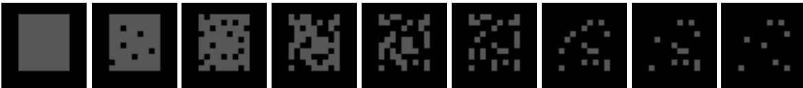
Figure 2: Temporal color change illustrated by frame sequence. Temporal correlogram captures the dispersion of the color element whereas histogram does not.
