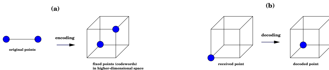
Figure 3: (a) Encoding the two points in \{0, 1\} by mapping them to two well-separated fixed points in \{0, 1\}^3 . (b) Decoding involves selecting the closest fixed point to the point received. This simple code is robust to a single corruption between the encoding and decoding steps.
